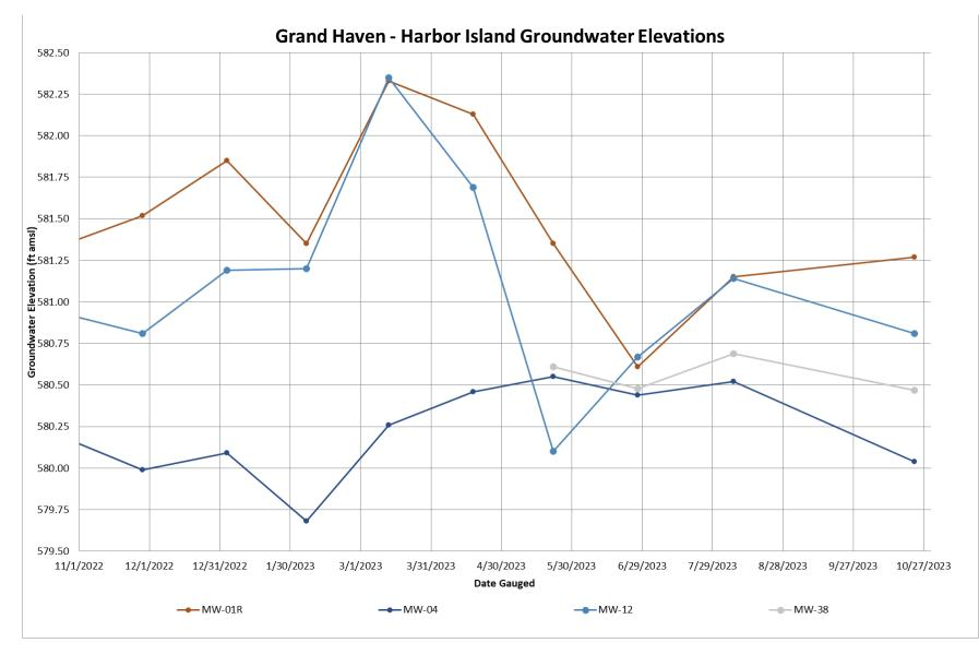
Figure 5. Hydrograph of Monitoring Wells South of Unit 3A/B Impoundment
