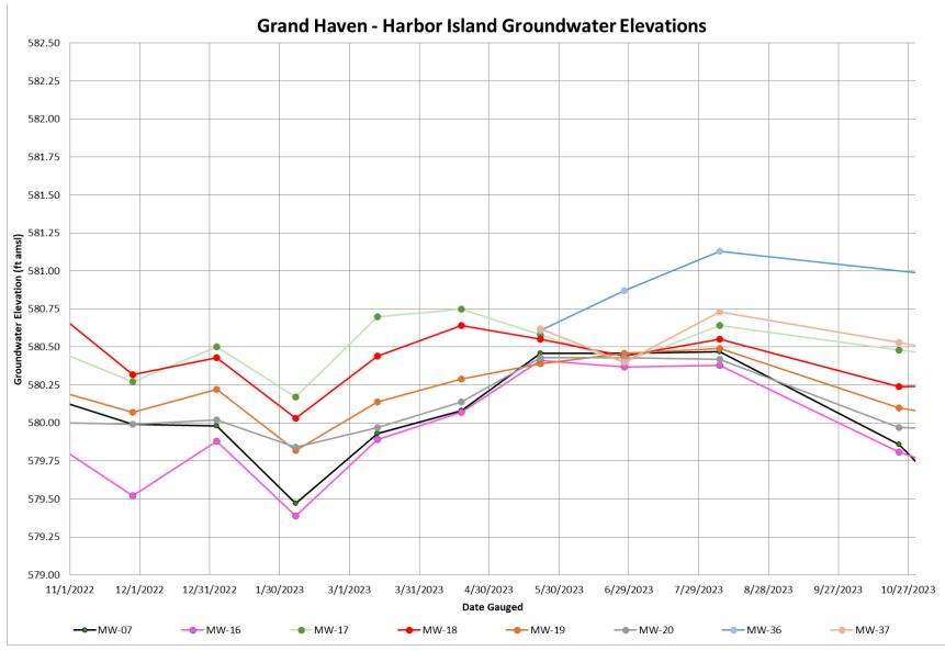
Figure 3. Hydrograph of Monitoring Wells South of Units 1/2 Impoundment
