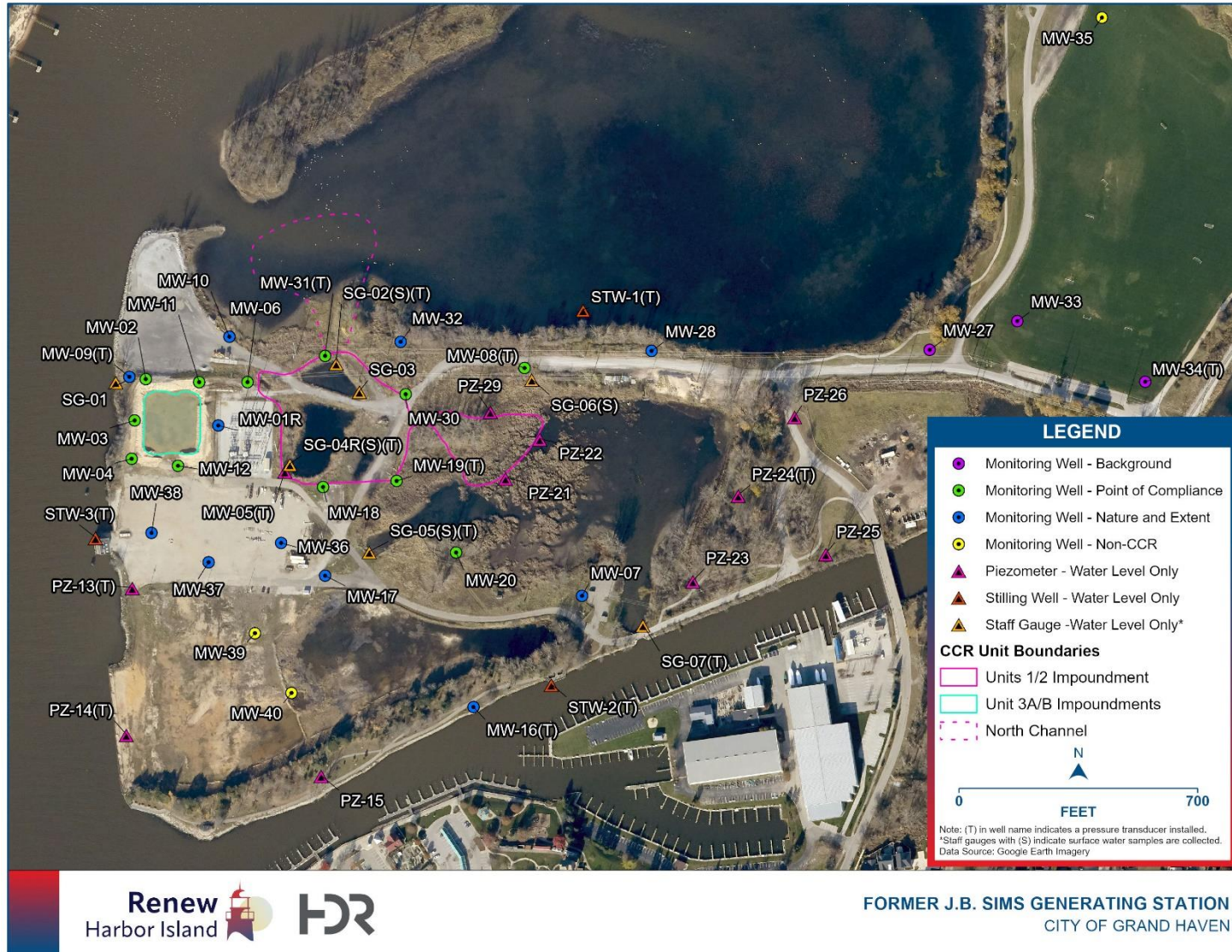
Figure 2 | Former J.B. Sims CCR Units and Monitoring Wells
